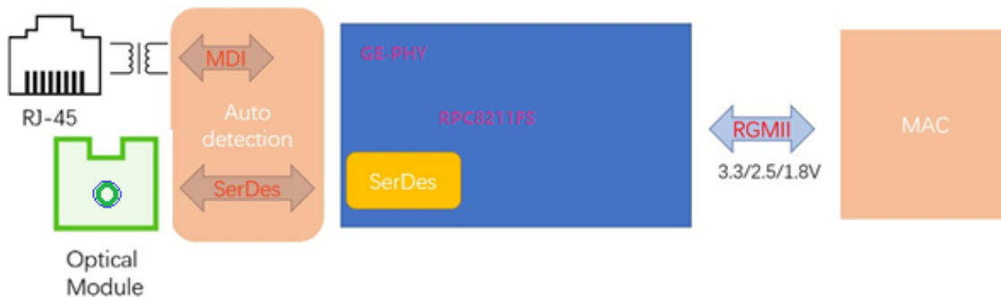
Figure 5. UTP/Fiber to RGMII Application
